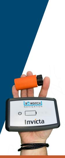
The Invicta 3 device is a combined GPS/GNSS receiver and AIS transceiver. It is used in pairs as an integral part of a portable pilot unit. Pairs of Invicta 3's are swappable, allowing one to charge inside the wheelhouse while the other provides a position on the bridge wing. The Invicta 3 connects by Wi-Fi, Bluetooth, or USB. It is compatible with all standard PPU software and computers. The Invicta 3 works with Windows computers or iPad tablets.
